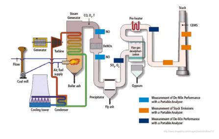
Many power plants use CEMS (Continuous Emissions Monitors) to analyze the total emissions being released from the stack of the power boiler. This information alone is not sufficient to pinpoint any deficiencies in the De-NOx system.
